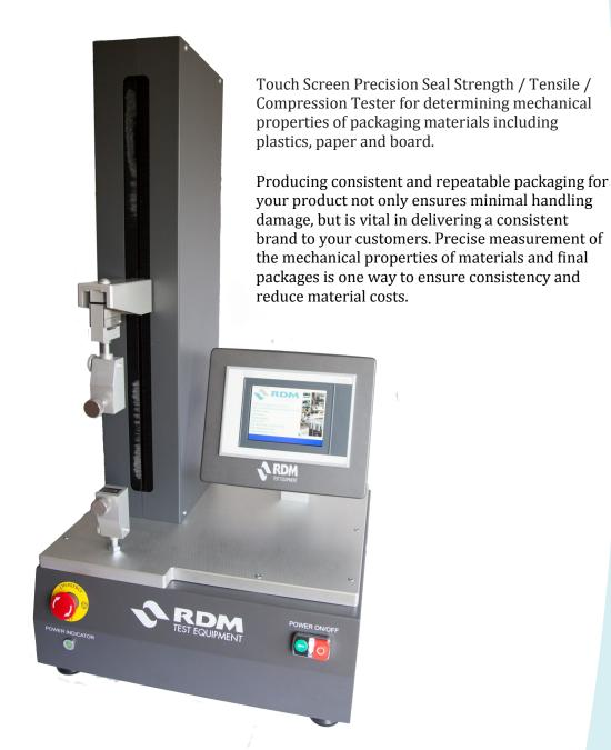
Accuracy and versatility in testing is vital, and the SST-3XS provides the technology and range of options to deliver for your specific needs. An intelligent controller and touch screen user interface stores multiple settings for later recall, and controls settings to ensure calibrated accuracy to international testing standards.
